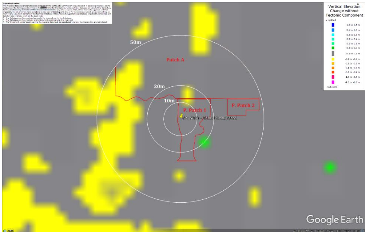
Figure 37: Ground surface subsidence without tectonic component for June 2011 Earthquake according to the LiDAR DEM.
